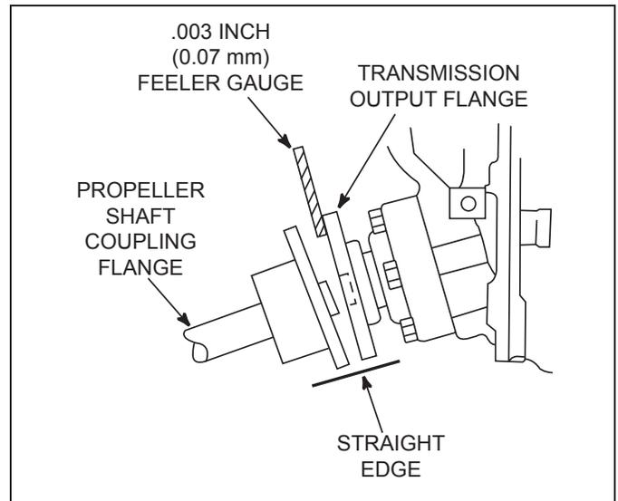
**Figure 11-30** Angular Alignment
