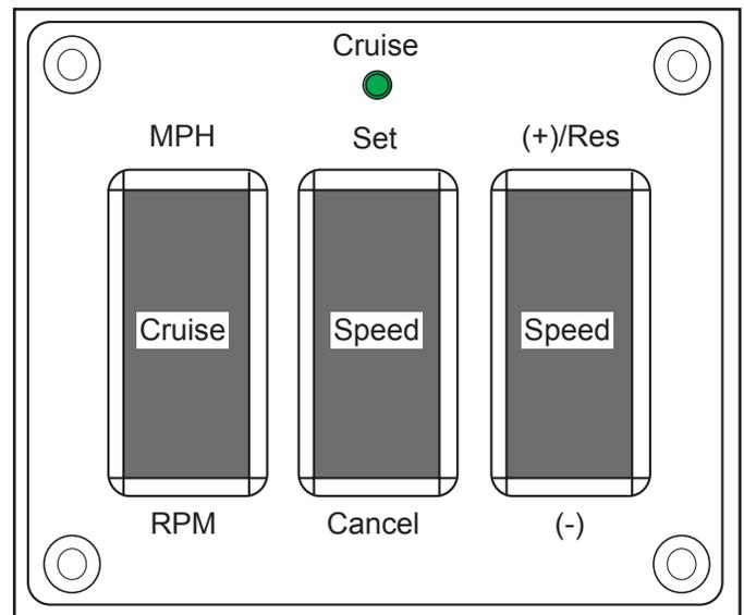
**Figure 5-4** Challenger Basic Cruise Control Panel (Typical)
