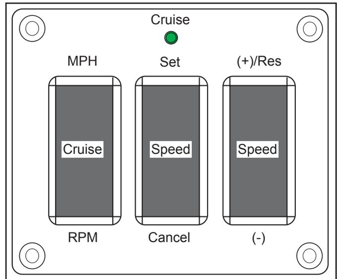
**Figure 5-3** Challenger Basic Cruise Control Panel (Example)
