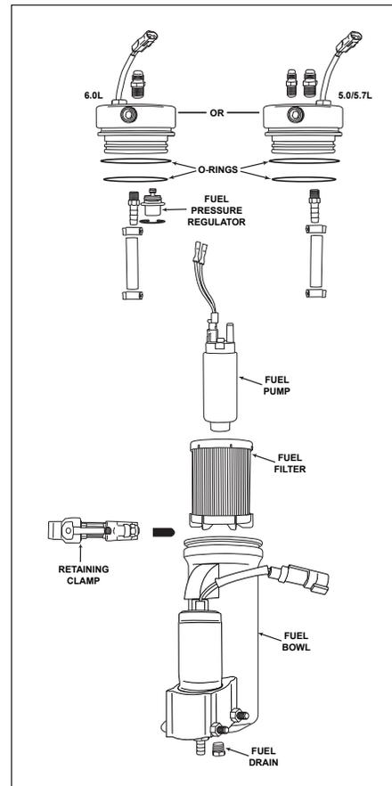
**Figure 11-15** Fuel Control Cell (FCC) - Clamp-on Canister (Typical)
