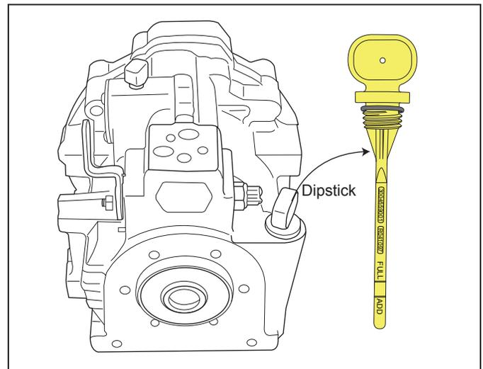
**Figure 11-2** 80 Series Transmission Dipstick and Location
