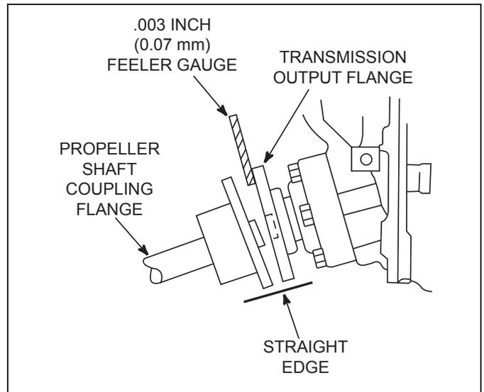
**Figure 11-26** Angular Alignment
