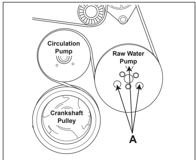
**Figure 11-20** 6.0L / 6.2L Raw Water Pump Removal
