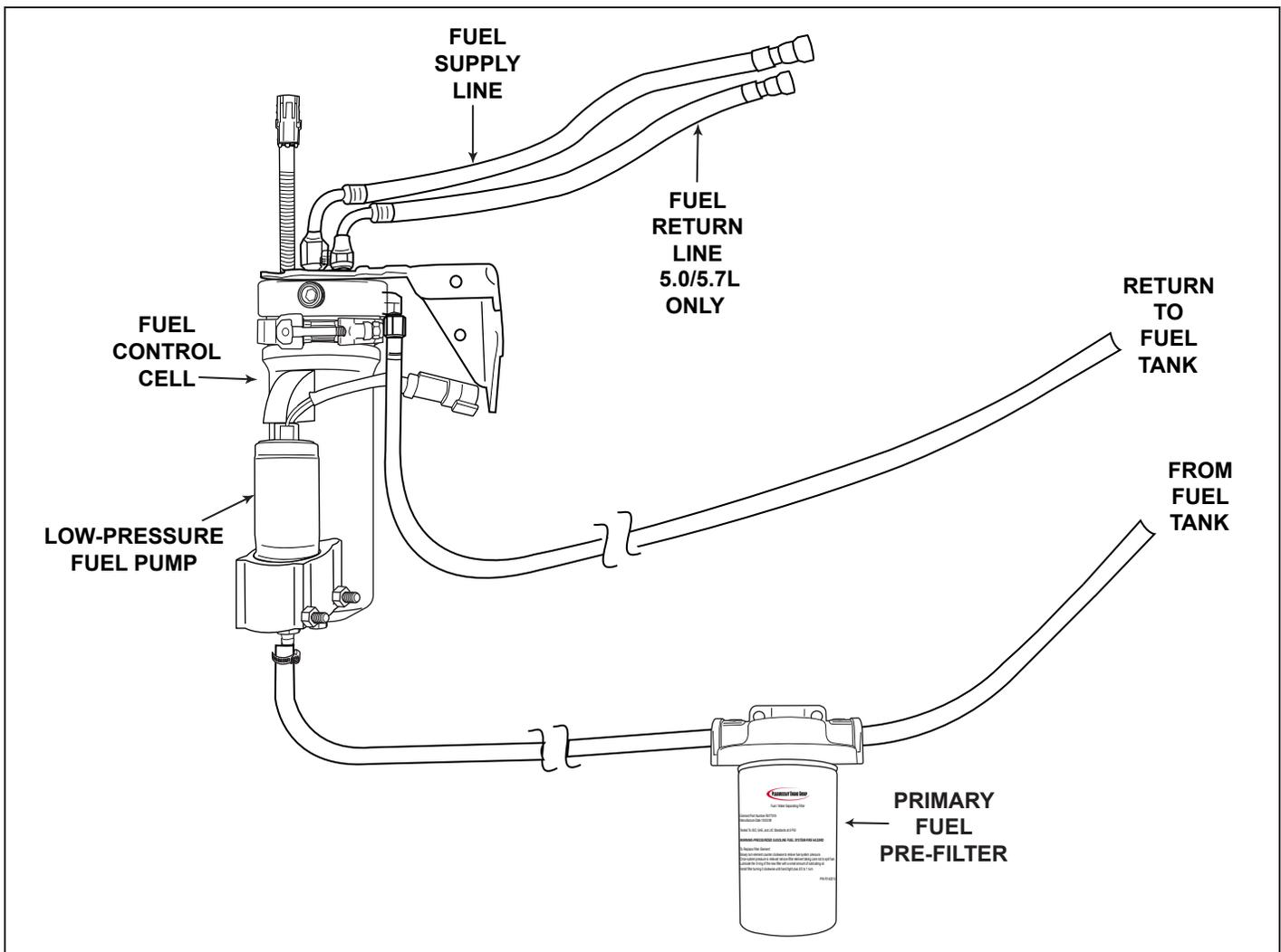
**Figure 11-14** Fuel Control Cell (FCC) Fuel System (Typical)
