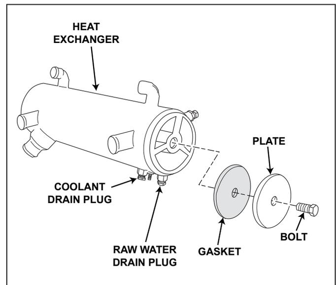
**Figure 11-13** Heat Exchanger and End Plate Removal (Typical)
