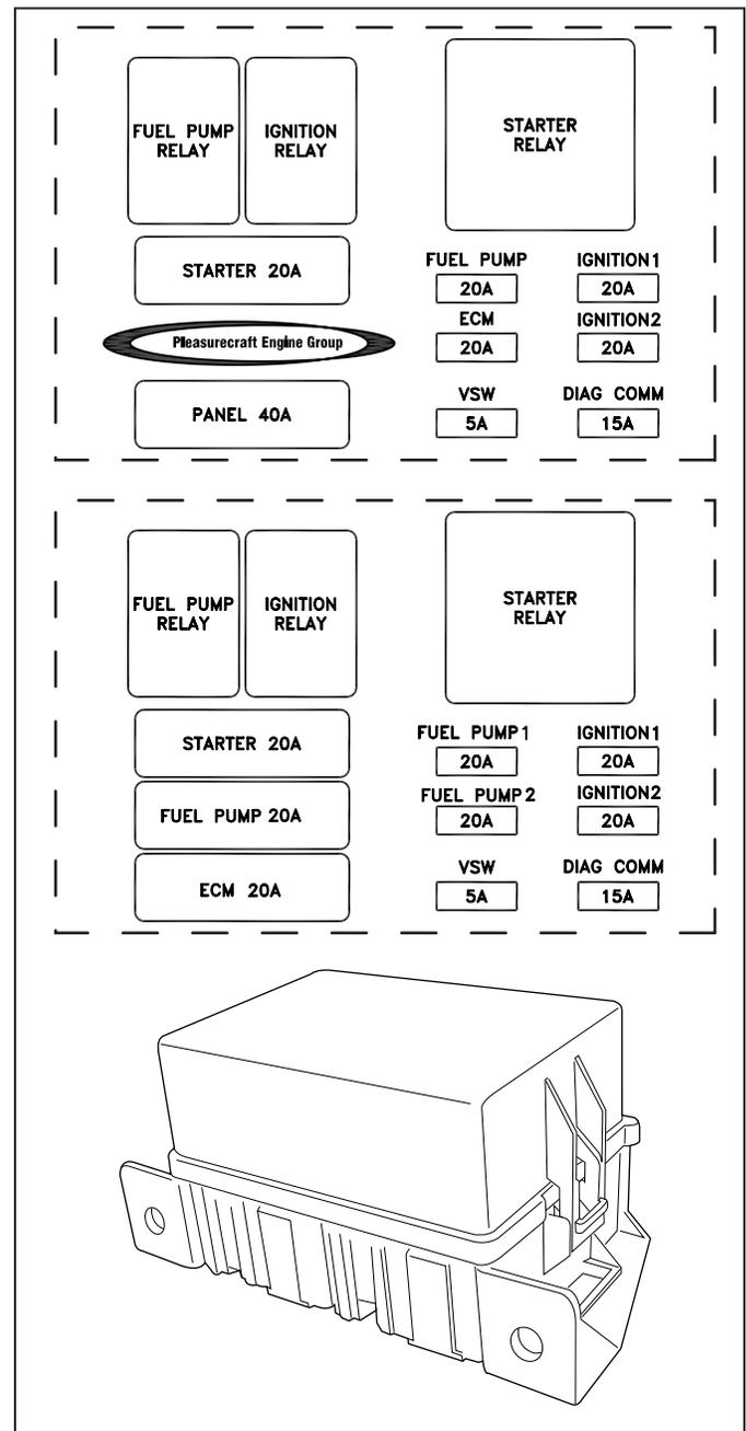
Figure 11-5 (Typical) Electrical System Relay and Fuse Block
