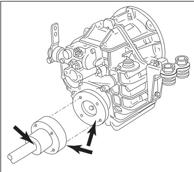
**Figure 11-28** Shaft Mating Surface Check - 8 Degree Down Angle
