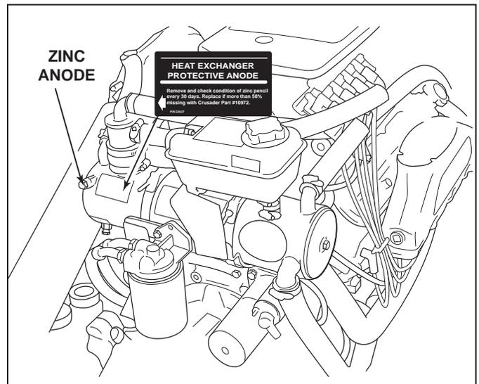
**Figure 11-7** Zinc Anode Location 8.1L F.W.C. Heat Exchanger
