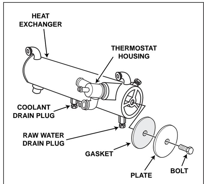
**Figure 11-12** Heat Exchanger and End Plate Removal (Typical)
