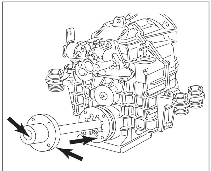
**Figure 11-29** Shaft Mating Surface Check - "V" Drives
