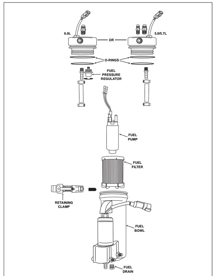
Figure 11-15 Fuel Control Cell (FCC) - Clamp-on Canister (Typical)
