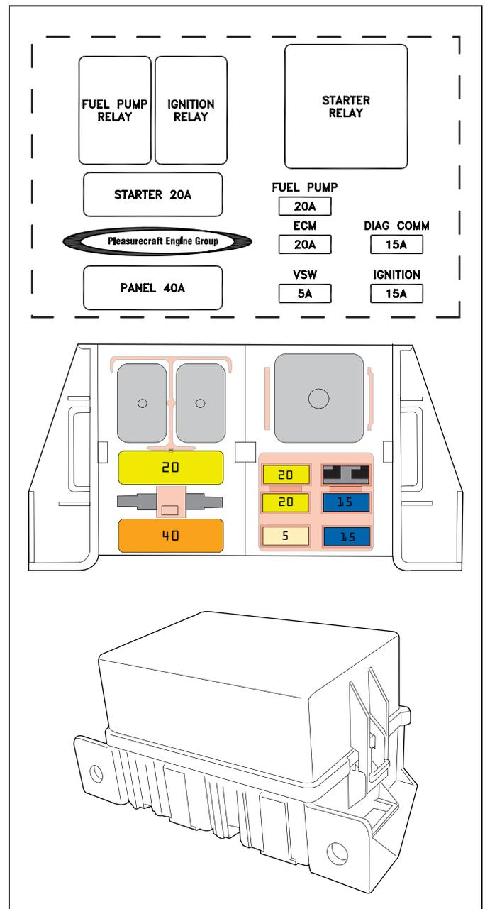
Figure 11-6 Electrical System Relay and Fuse Block
