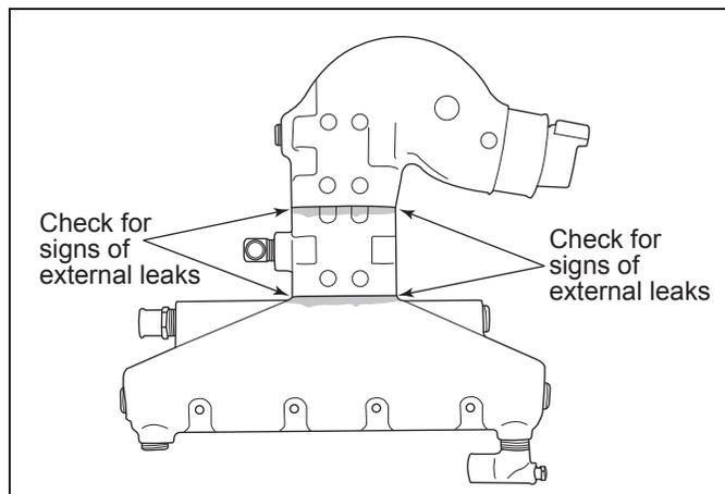
**Figure 5-2A** Water Leaks
