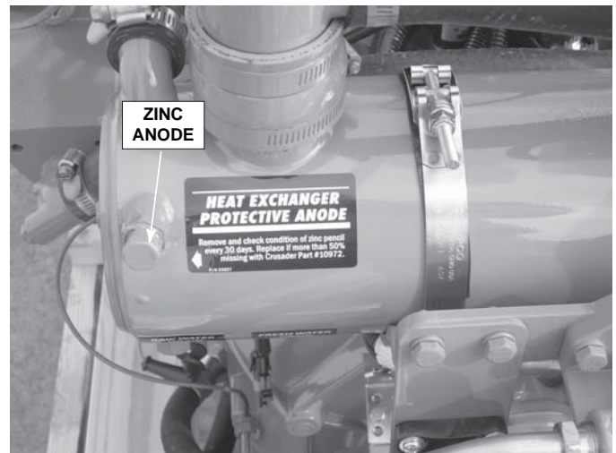
Figure 10-7 Zinc Anode Location F.W.C. Heat Exchanger (Typical)
